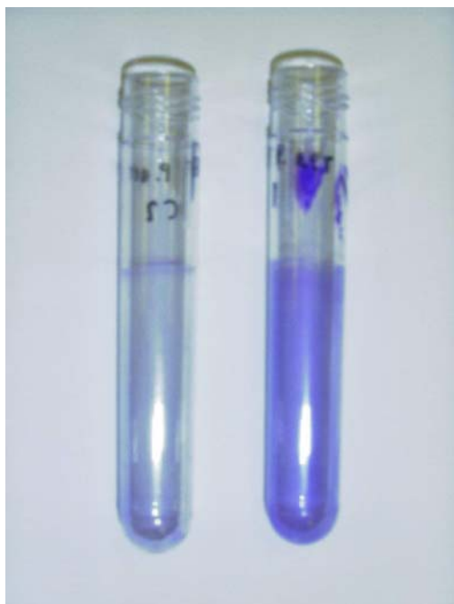
Fig 4 Biofilm formation of P. aeruginosa growing nutrient broth in tubes treated with the Mark 1 device (left) and the control tubes (right).
